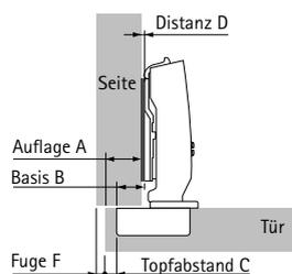
$$\text{Distanz D} = \text{C} + \text{B} - \text{A}$$
