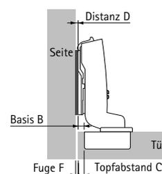
$$\text{Distanz D} = \text{C} + \text{B} + \text{F}$$
