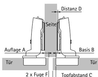
$$\text{Distanz D} = \text{C} + \text{B} - \text{A}$$
